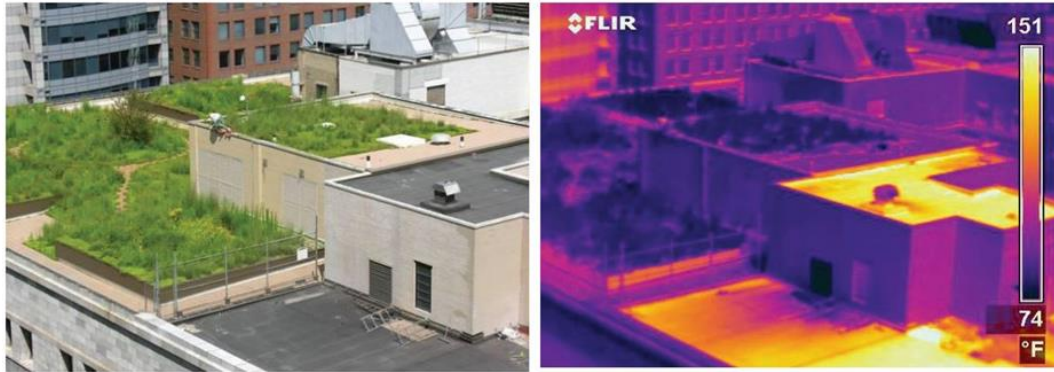
Figure 3.27 Temperature differences between conventional and green roof in Chicago City Hall
