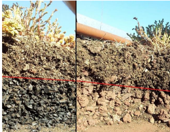
Figure 3.23 Granular porous materials
